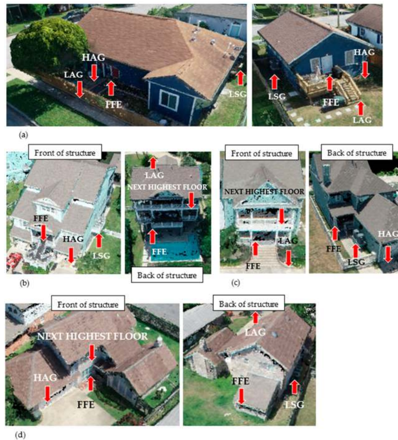
Figure 3. Interpretations of measures derived from the residential community models produced within Pix4D. Example shown in tiles (a) Silk-stocking district, (b) Laffite's Cove, (c) Evia, (d) Campeche Cove.
